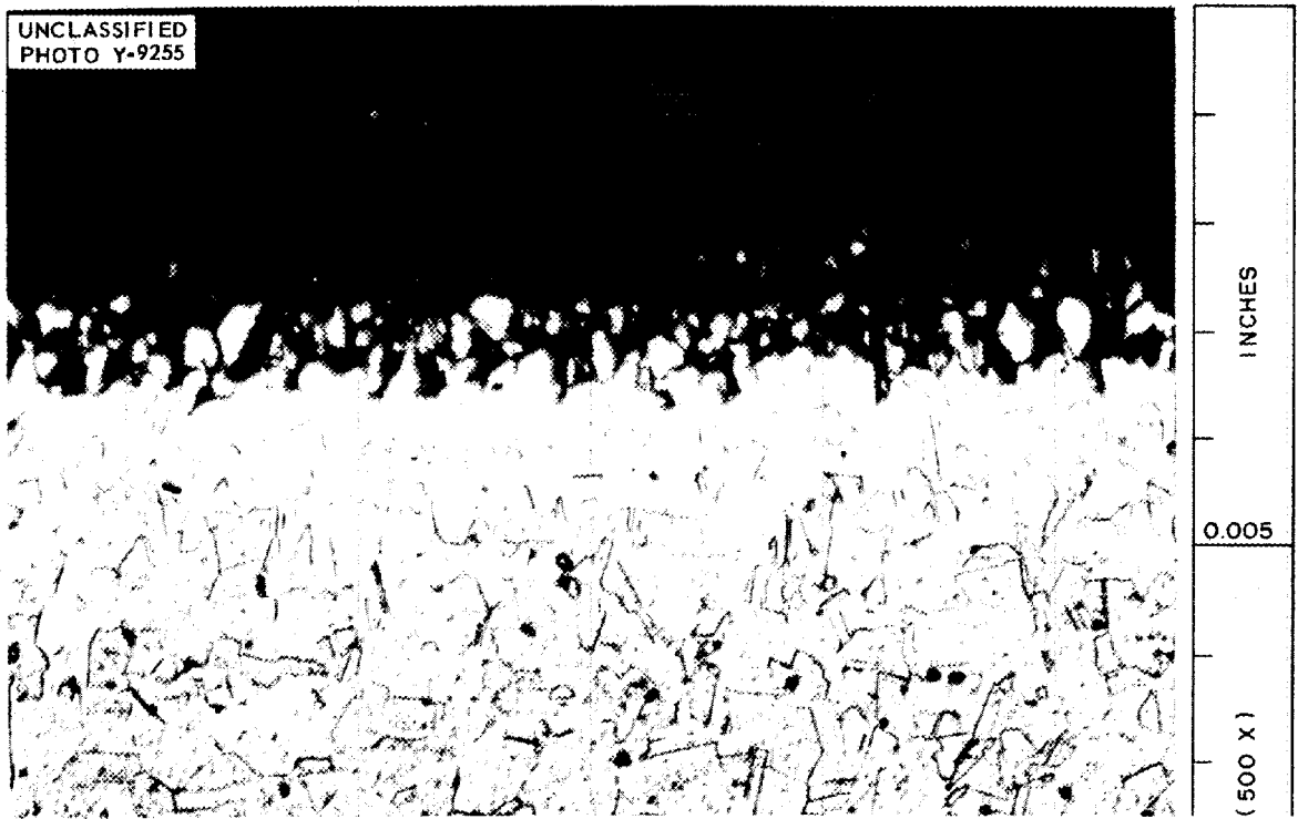
Fig. 7.9. Corrosion of Type 347 Stainless Steel by Lead in Quartz Thermal Convection Loop After 140 hr at 800°C. 500X
