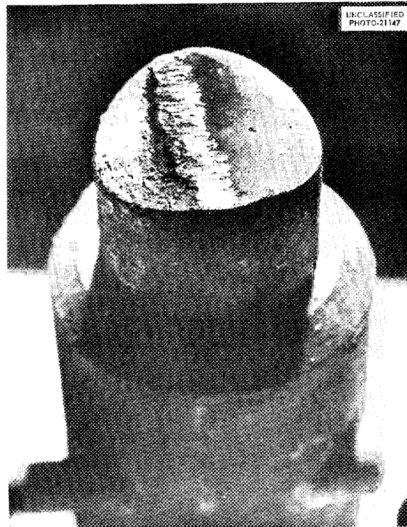
Fig. 2.7. Metallic Iron Buildup of Chrome Carbide Bearing Material Tested at 1200°F for 2 hr in Fluoride Mixture NaF-ZrF 4 -UF 4 (50-46-4 mole %).
