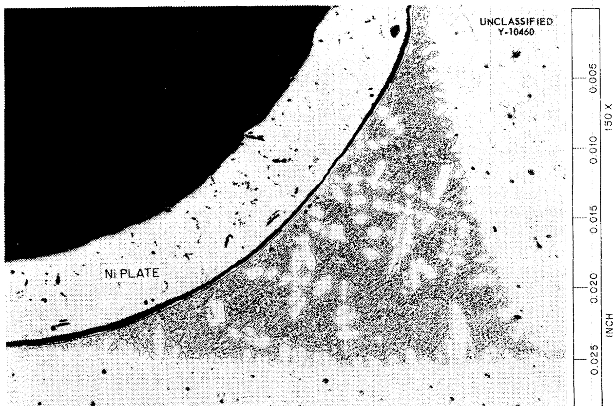
Fig. 6.5. Inconel T-Joint Brazed with 90% Ni-10% P Alloy after Exposure for 100 hr at 1500°F in NaF-ZrF 4 -UF 4 (50-46-4 mole %). Specimen nickel plated after testing to preserve the edge during polishing. Etched with aqua regia. 150X
