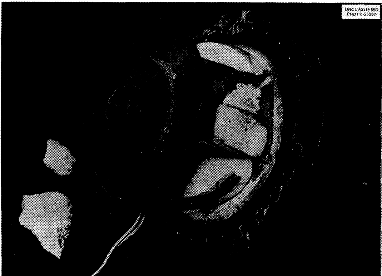
Fig. 2.4. Zirconium Fluoride Crystal Formation in Sump Pump Used to Circulate \text{NaF-ZrF}_4 for 1370 hr at 1200 to 1600°F.
