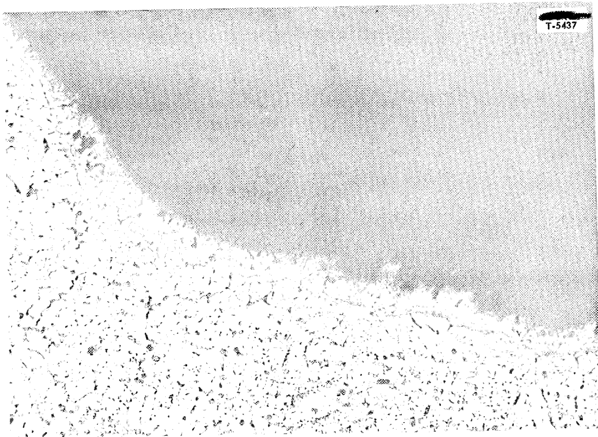
Fig. 5.10. Hot-Leg Surface and Weld Bead of a Hastelloy B Loop After Circulation of \text{NaF-ZrF}_4\text{-UF}_4 (50-46-4 mole %) for 500 hr at a Hot-Leg Temperature of 1500^\circ\text{F} . 250X.
