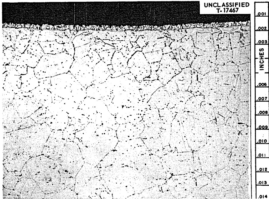
Fig. 2.1.6. Specimen Taken from Hot Leg of INOR-8 Forced-Circulation Loop 9354-5 at Point of Maximum Loop Temperature (1300°F). Loop was operated for 8938 hr with salt mixture \text{LiF}\text{-BeF}_2\text{-UF}_4 (62-37-1 mole %). Etchant: 3 parts \text{HCl} , 2 parts \text{H}_2\text{O} , 1 part 10% chromic acid. 250X.
