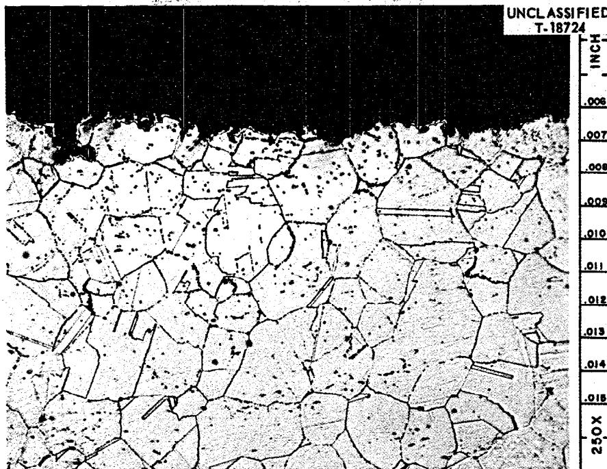
Fig. 2.1.4. Specimen Removed from INOR-8 Forced-Convection Loop 9354-1 at Point of Maximum Salt-Metal Interface Temperature (1300°F) Showing Maximum Attack Found. Loop operated for 14,563 hr with salt mixture \text{LiF}\cdot\text{BeF}_2\cdot\text{UF}_4 (53-46-1 mole %). Etchant: 3 parts \text{HCl} , 2 parts \text{H}_2\text{O} , 1 part 10% chromic acid.
