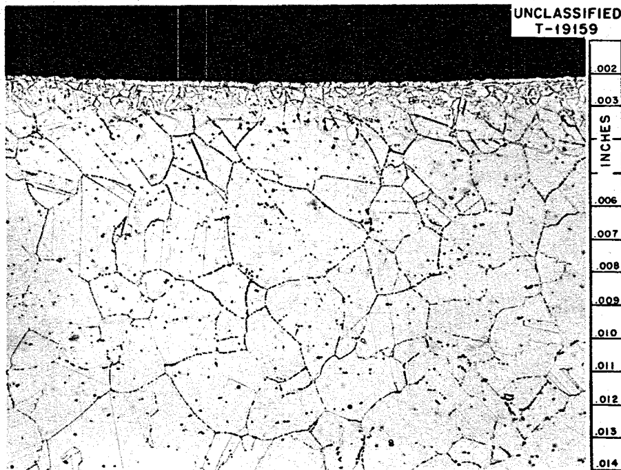
Fig. 4.1. Transverse Section of 15,000-hr Insert Removed from INOR-8 Forced-Convection Loop 9354-4. Etchant: 3 parts HCl, 2 parts H 2 O, 1 part 10% chromic acid. 250X.
