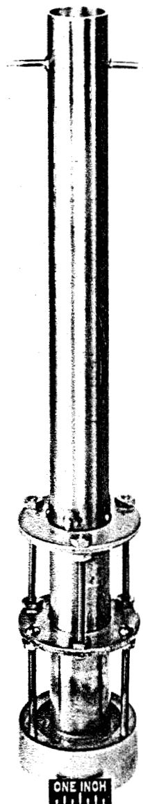
Fig. 4.2. Test Rig with Sump-Type Seal.
