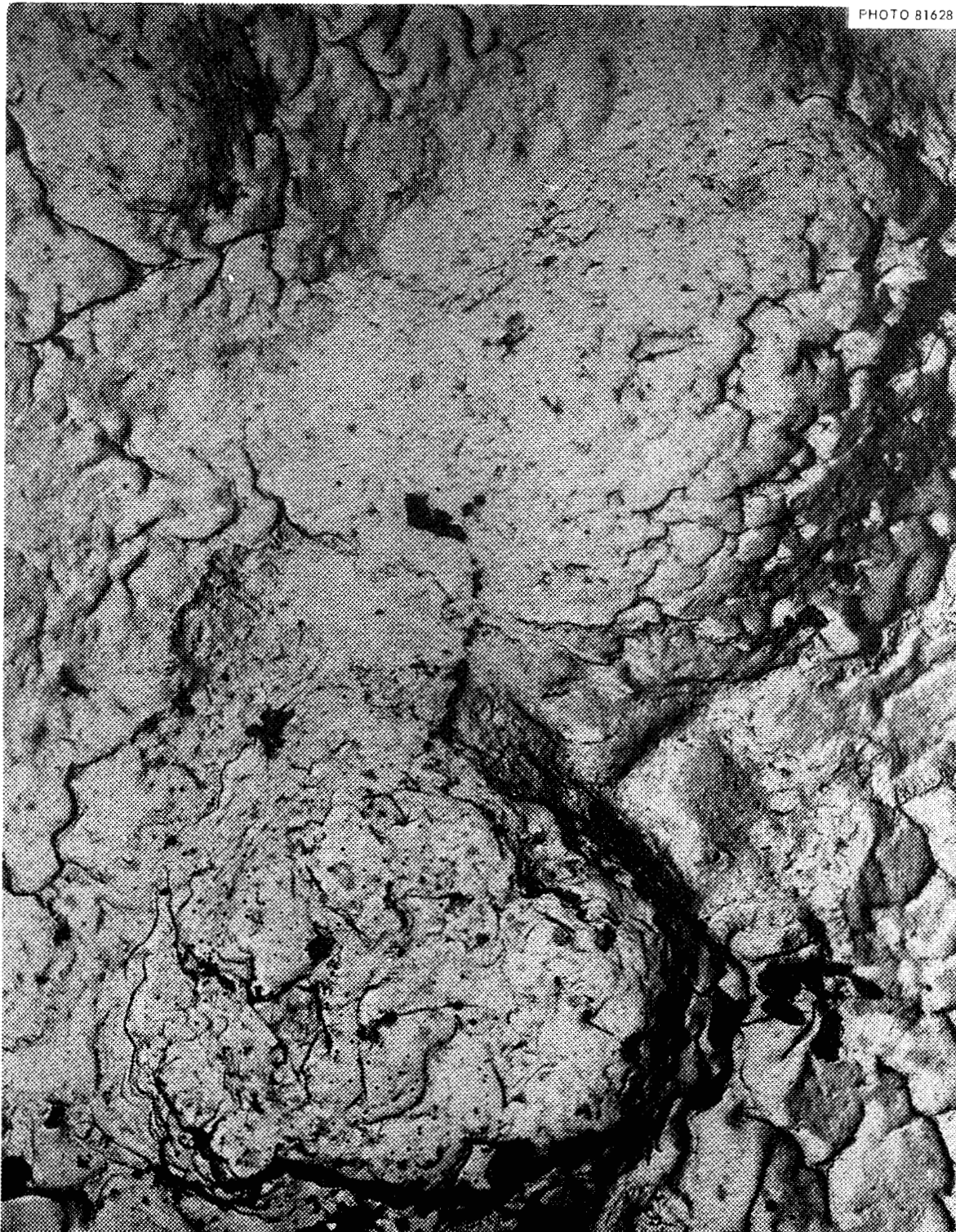
Fig. 12.2. Electron Micrograph of MgO of Density 3.4 \text{ g/cm}^3 and Grain Size 10 \mu Irradiated to a Fast-Neutron Dose of 1.2 \times 10^{21} Neutrons/cm 2 ( >1 \text{ Mev} ) at 150^\circ\text{C} at 32,000\times Magnification Showing General Deterioration and Small Cracks. Reduced 12.5%.
