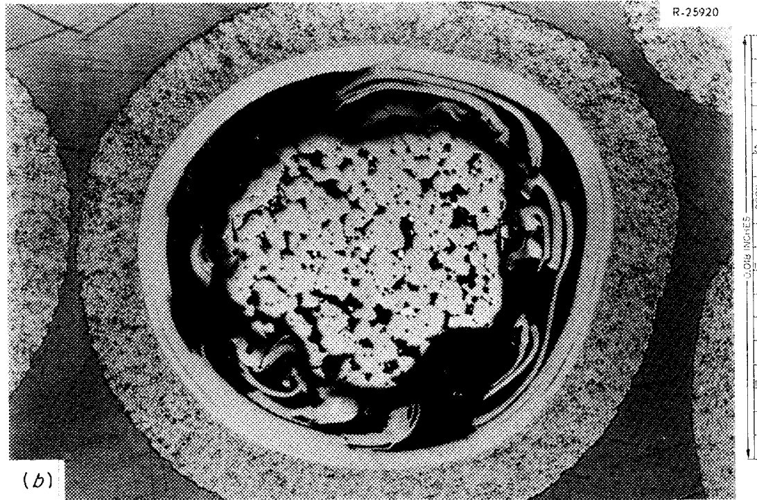
Fig. 10.2. Pyrolytic-Carbon-Coated Uranium Oxide Particles from Batch OR-298. Magnification 200 \times : (a) unirradiated; (b) irradiated to 28% burnup at 1400 ^{\circ} C in capsule A9-2.
