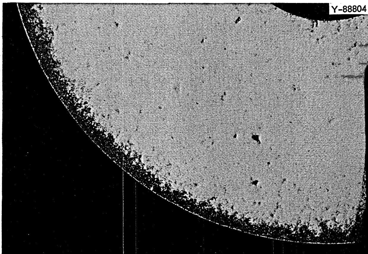
Fig. 18. Effectiveness of a Gas Impregnation Technique for Graphite Permeability Reduction as Evidenced by a Radiographic Method Employing Mercury Penetration. The light section, which is opaque to the x rays, has been penetrated by the mercury. The graphite surface where permeability reduction has been effected remains translucent to the radiation.
