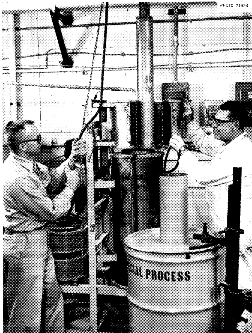
Fig. 26. Fluoride Production for MSRE – Storage Container and Holder for Enriched Fuel Concentrate Mixture.
