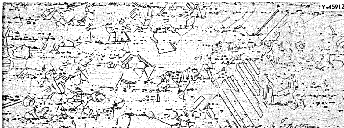
Fig. 2. As-Received INOR-8 Heat 5075. Etchant: aqua regia. 100X.
