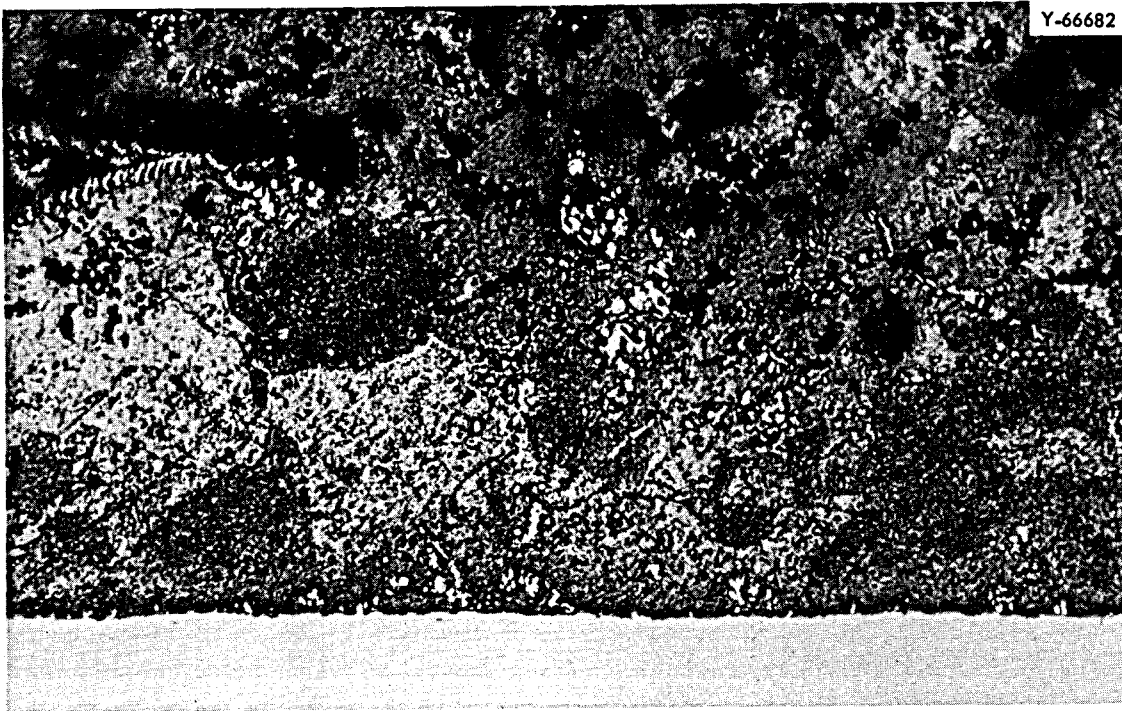
Fig. 8. Niobium Crystals Found in Cold Leg of Nb-1% Zr Loop Which Operated Over 5000 hr at 1400°F and a \Delta T of 400°F. Unetched. 250x.
