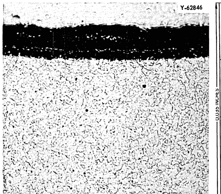
Fig. 6. Section Through Hot Leg of 2 1/4 Cr Lead Loop Which Operated for 5156 hr with a Hot-Leg Temperature of 1100°F and a \Delta T of 200°F. The attack consisted of uniform surface removal.
