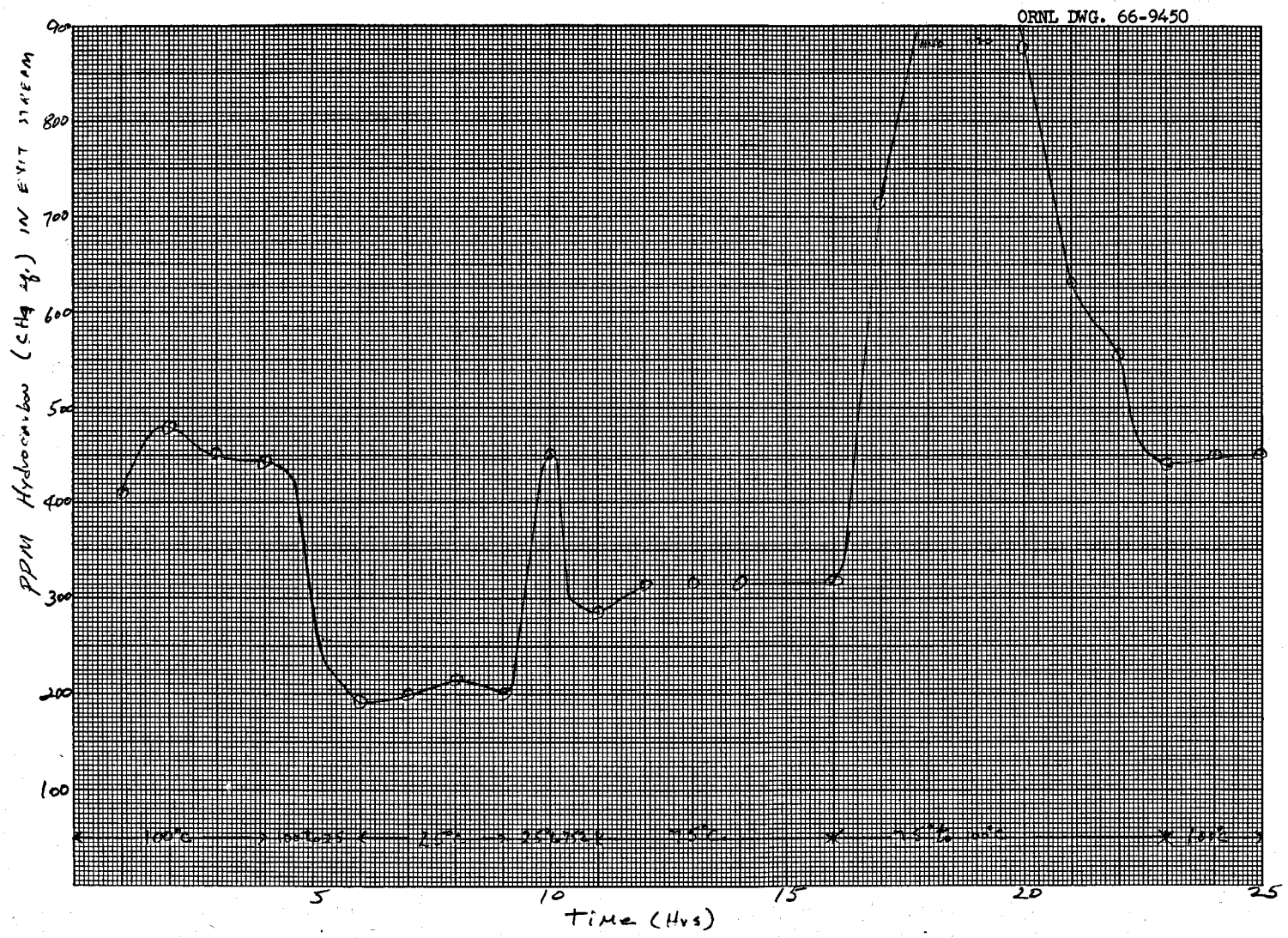
Fig. 5. Hydrocarbon Adsorption on Charcoal at 25°C, 75°C, and 100°C.
