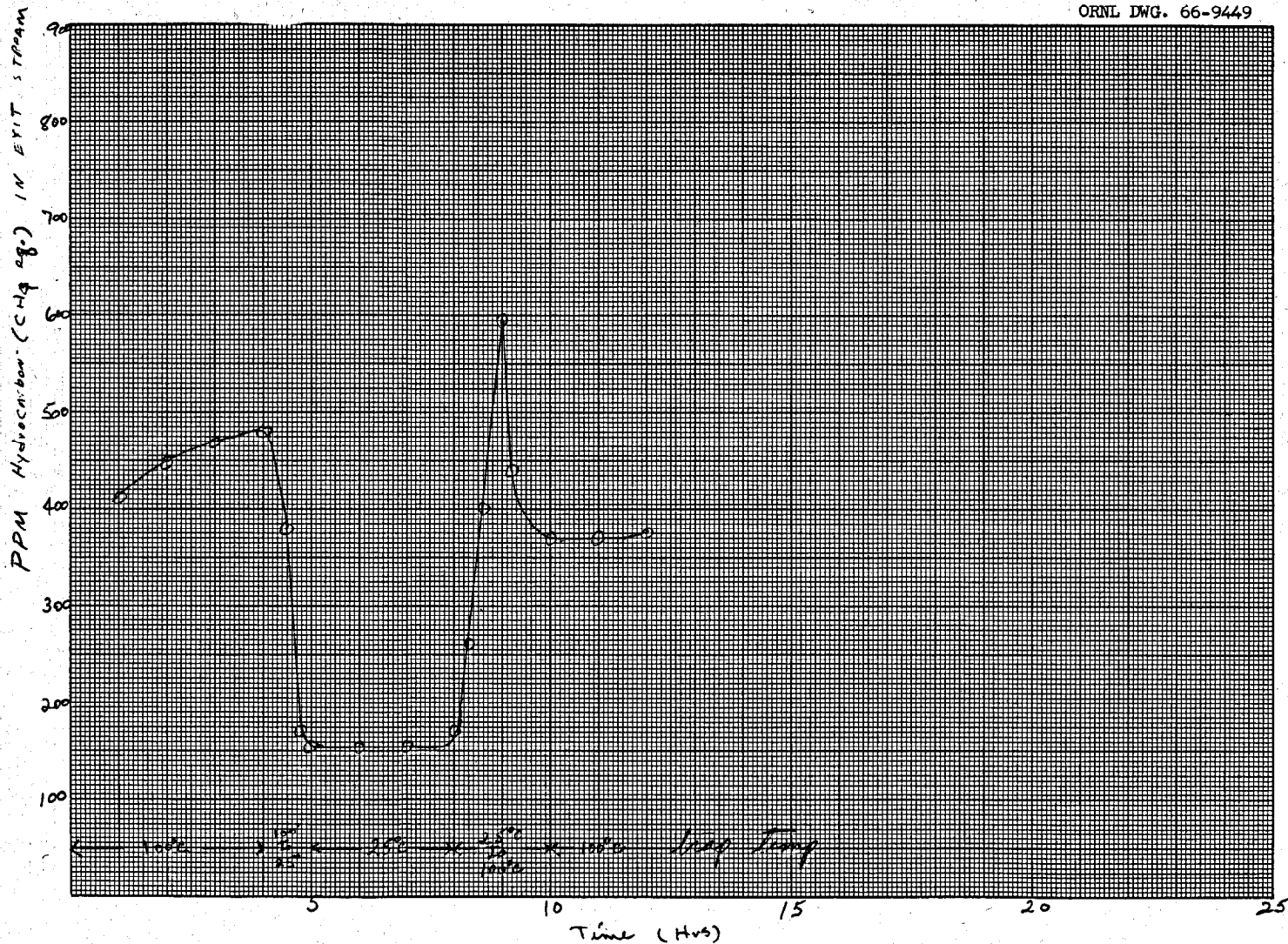
Fig. 4. Hydrocarbon Adsorption on Charcoal at 25°C and 100°C
