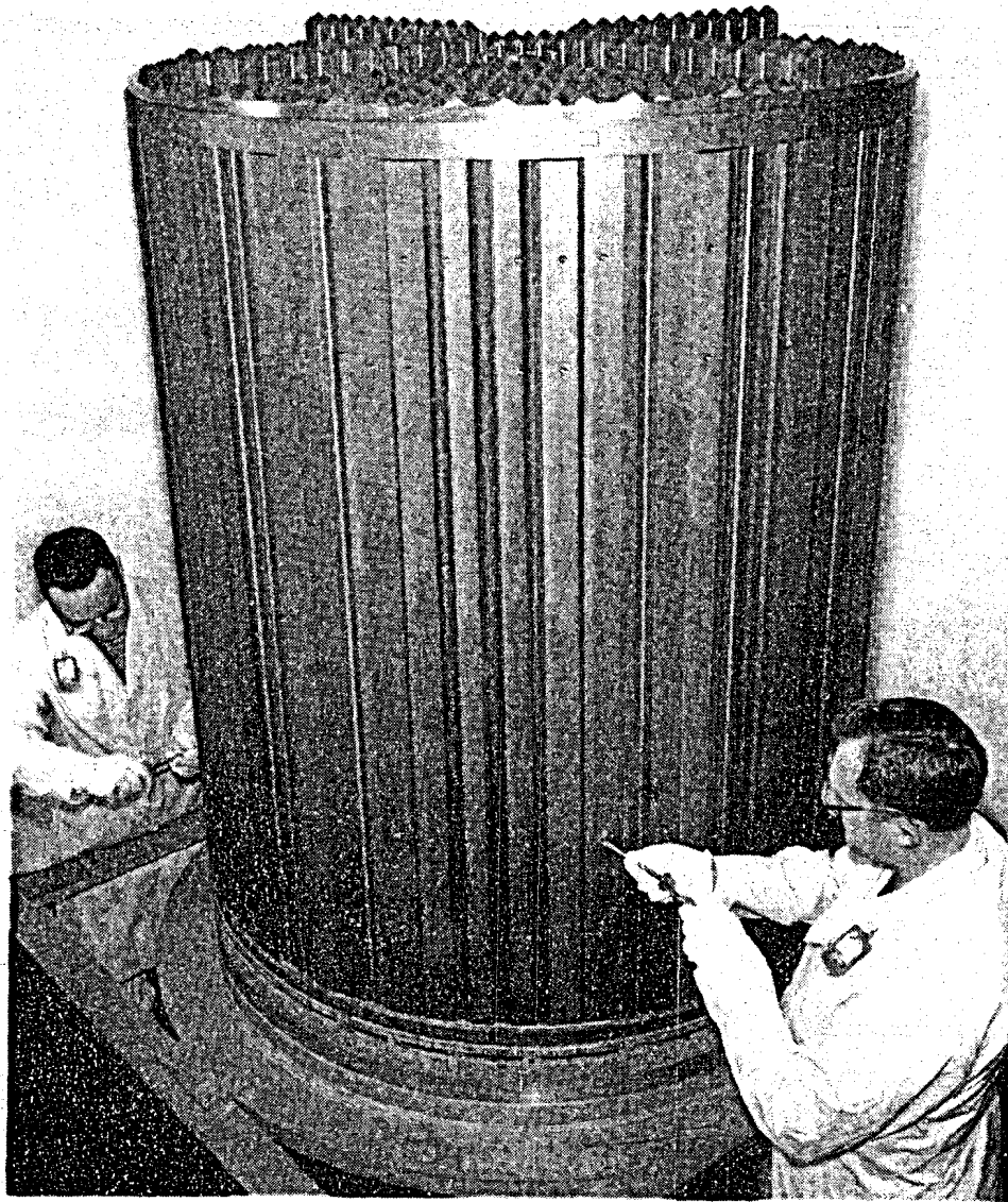
Fig. 25. Anisotropic, Needle-Coke Graphite Grade CGB Being Assembled for MSRE Core.
