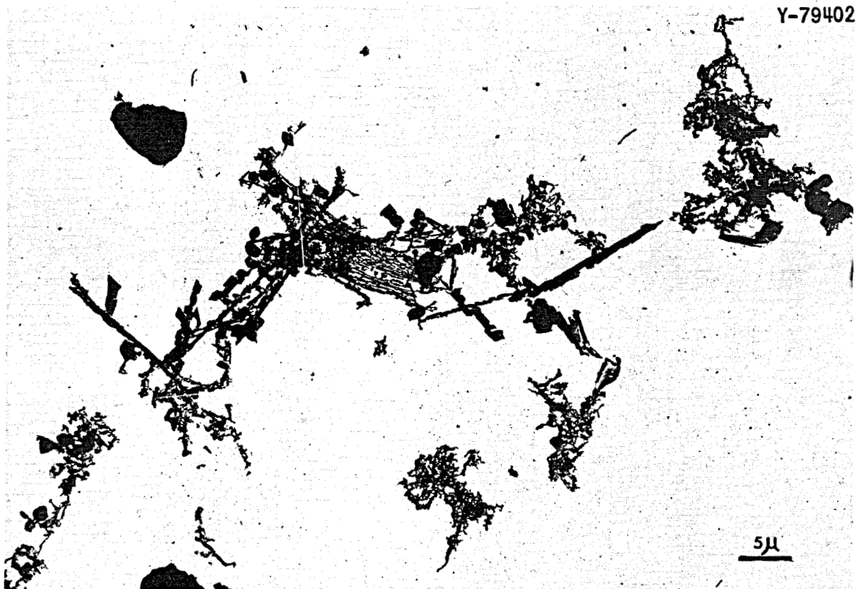
Fig. 35. Extraction Replica From Surveillance Specimen, Heat 5081.
