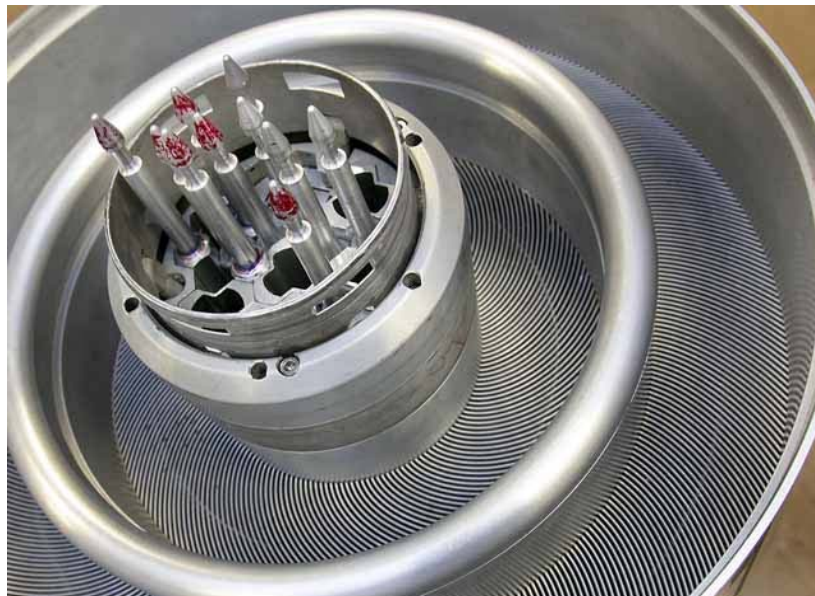
Fig. 49. HFIR fuel element with target rods in the flux trap. (ORNL Photo 2008-P01868)
