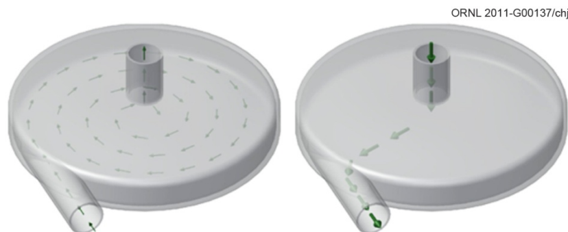
Fig. 5.9. Forward (right) and reverse (left) operation of a vortex diode.
