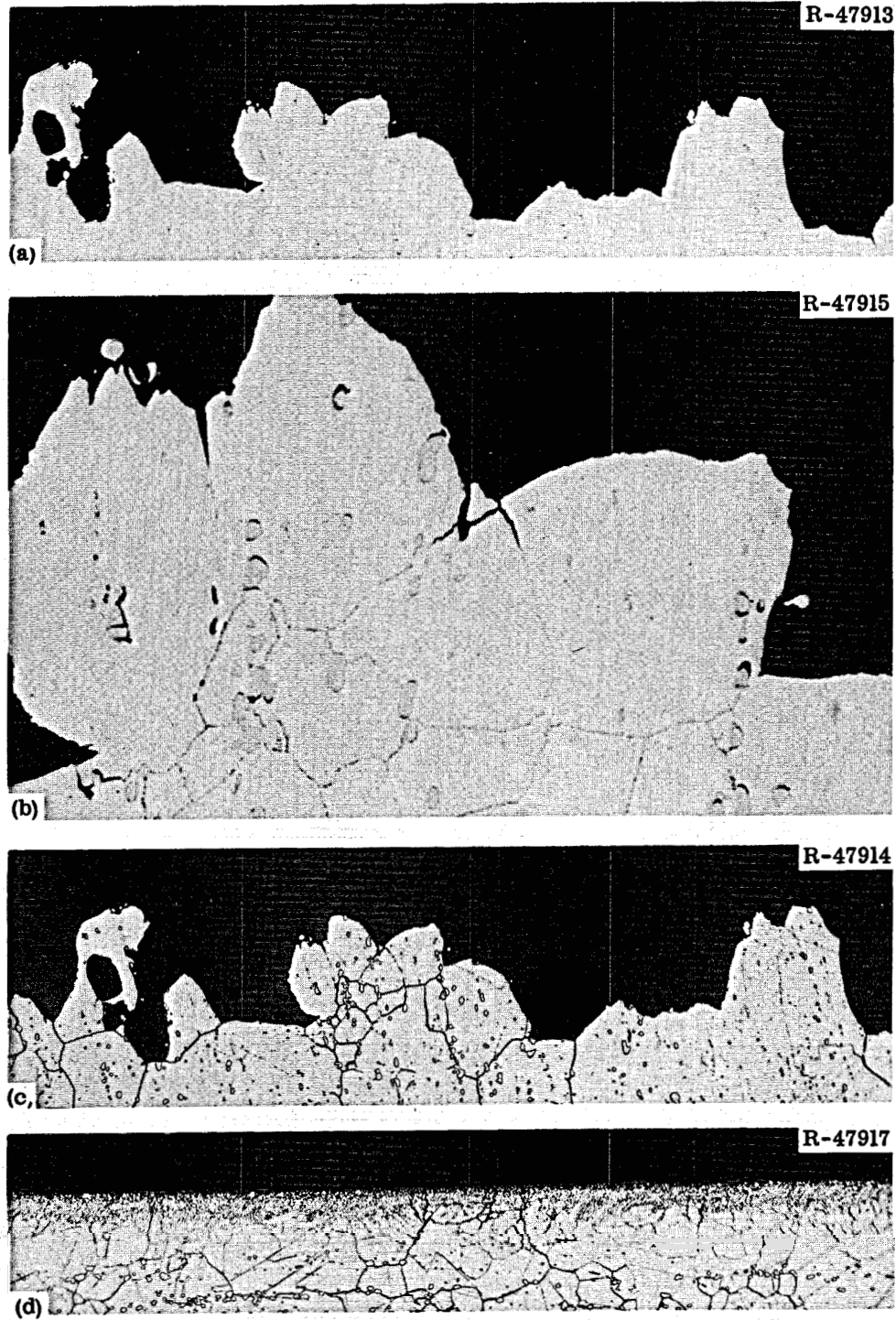
Fig. 43. Photomicrographs of a Hastelloy N (Heat 5085) Sample Exposed to Fluoride Salt in the MSRE for 15,289 hr at 650°C and Then Tested at 650°C and a Strain Rate of 0.002 min -1 . Thermal fluence was 9.4 \times 10^{20} neutrons/cm 2 . (a) Fracture, as polished. 100X. (b) Fracture, as polished. 500X. (c) Fracture, etched. 100X. (d) Edge of stressed portion, etched. 100X. Etchant: aqua regia. Reduced 14.5%.
