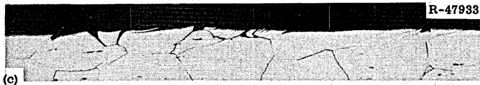
Fig. 54. Photomicrographs of a Hastelloy N (Heat 67-504) Sample Exposed to Fluoride Salt in the MSRE for 9789 hr at 650°C and Tested at 25°C. 100X. (a) Fracture, as polished. (b) Fracture, etched. (c) Edge of stressed portion, etched. Etchant: aqua regia. Reduced 10%.
