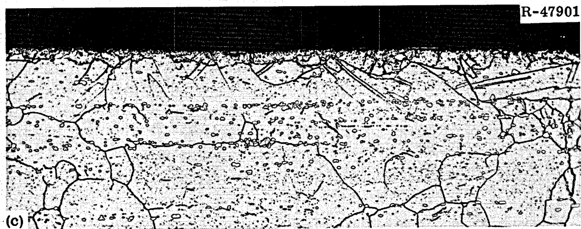
Fig. 37. Photomicrographs of a Hastelloy N (Heat 5085) Sample Tested at 650^{\circ}\text{C} at a Strain Rate of 0.002 \text{ min}^{-1} . Sample had been irradiated to a thermal fluence of 2.6 \times 10^{19} neutrons/cm 2 while being exposed to the cell environment at 650^{\circ}\text{C} for 20,789 hr. 100X. (a) Fracture, as polished. (b) Fracture, etched. (c) Edge of stressed portion, etched. Etchant: aqua regia.
