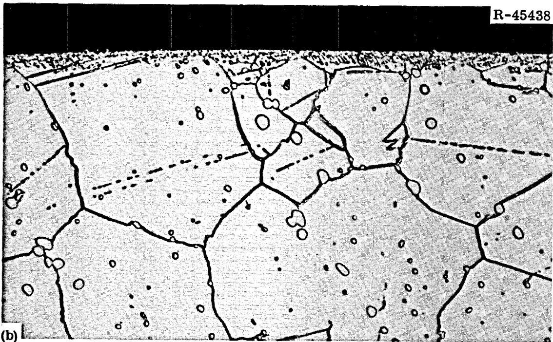
Fig. 4. Photomicrographs of Hastelloy N (Heat 5085) Surveillance Specimens Exposed to Fuel Salt for 15,289 hr at 650°C. 500X. (a) Unetched. (b) Etched (glyceria regia) photomicrographs showing shallow reaction layer near surface.
