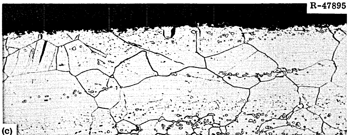
Fig. 36. Photomicrographs of a Hastelloy N (Heat 5085) Sample Tested at 25°C at a Strain Rate of 0.05 min -1 . Sample had been irradiated to a thermal fluence of 2.6 \times 10^{19} neutrons/cm 2 while being exposed to the cell environment at 650°C for 20,789 hr. 100X. (a) Fracture, as polished. (b) Fracture, etched. (c) Edge of stressed portion. Etchant: aqua regia.
