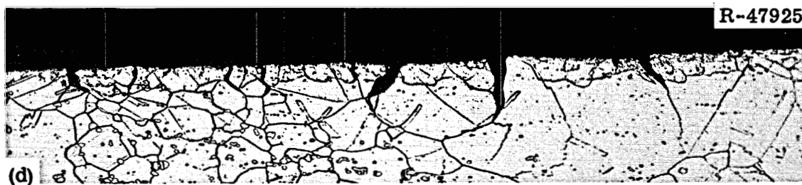
Fig. 41. Photomicrographs of a Hastelloy N (Heat 5085) Sample Exposed to Fluoride Salt in the MSRE for 15,289 hr at 650°C and Then Tested at 25°C. Thermal Fluence was 9.4 \times 10^{20} neutrons/cm 2 . (a) Fracture, as polished. 100x. (b) Fracture, as polished. 500x. (c) Fracture, etched. 100x. (d) Edge of stressed portion, etched. 100x. Etchant: aqua regia.
