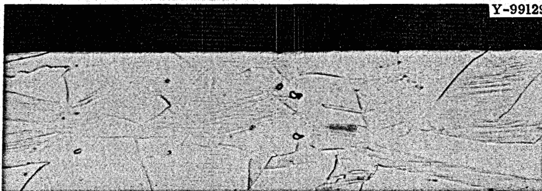
Fig. 8. Hastelloy N Exposed to \text{NaBF}_4 -8 mole % NaF for 1200 hr at 760°C. Etched with glyceria regia, 500x.
