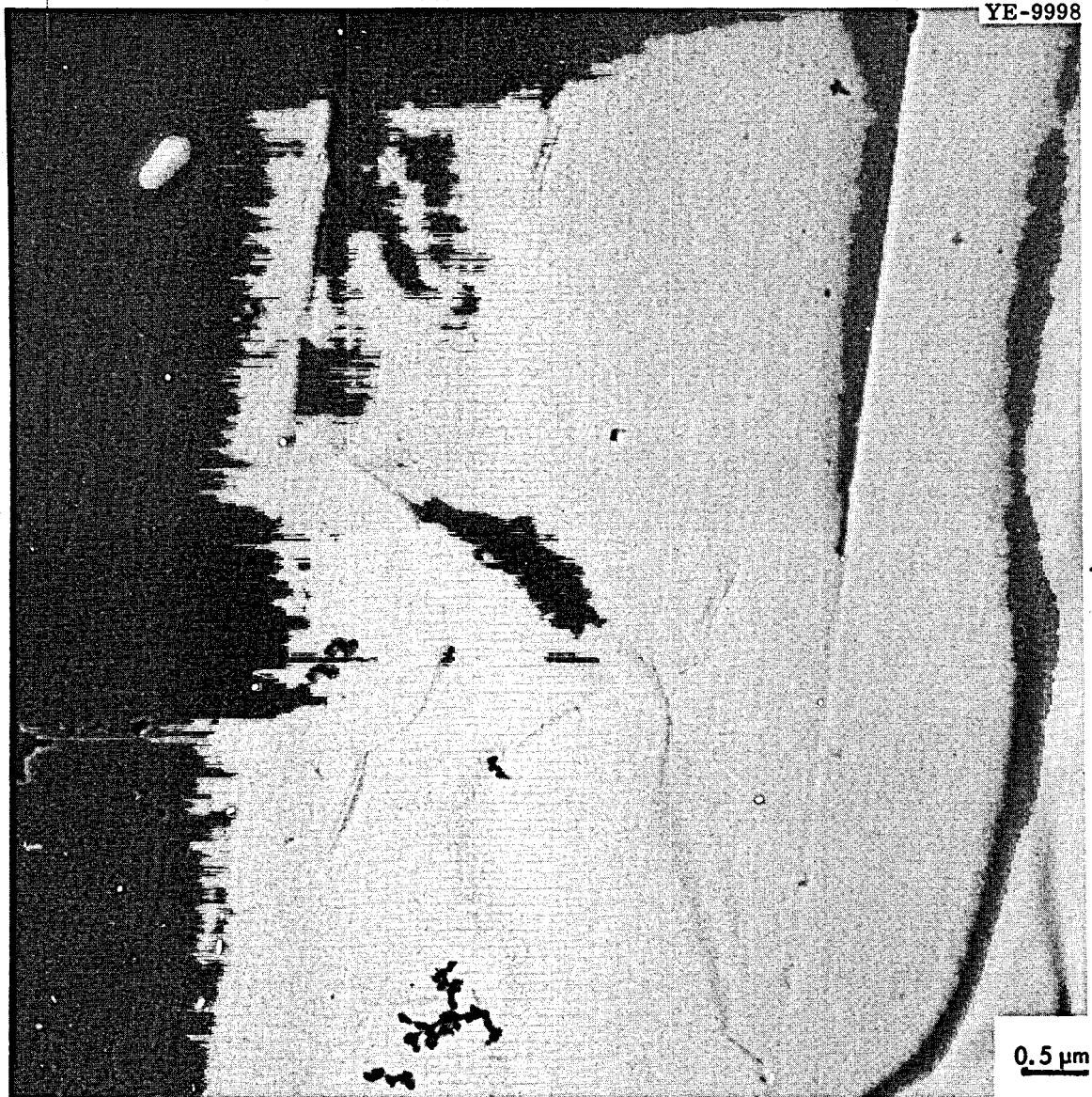
Fig. 8. Transmission Electron Micrograph of Hastelloy N (Heat 5085) Exposed to the MSRE Core for 22,533 hr at 650°C. Irradiated to a thermal neutron fluence of 1.5 \times 10^{21} neutrons/cm 2 and a fast neutron fluence of 3.1 \times 10^{20} neutrons/cm 2 (> 1.22 Mev). The white spots are helium bubbles that are located on a twin boundary. 25,000X. Reduced 16%.
