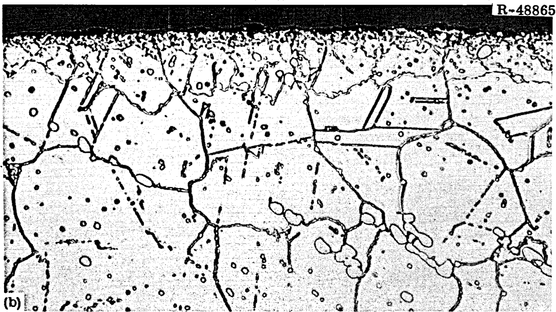
Fig. 4. Typical Photomicrographs of Hastelloy N (Heat 5085) Exposed to the MSRE Core for 22,533 hr at 650°C. (a) As polished. (b) Etchant: glyceria regia. 500X.
