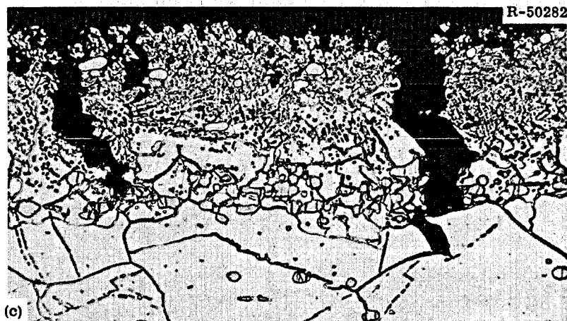
Fig. 5. Typical Photomicrographs of a Hastelloy N (Heat 5085) Sample Exposed to the MSRE Core for 22,533 hr at 650°C. The sample was bent in a vise. (a) As polished, tension side. (b) As polished, tension side. (c) Etched, tension side. (d) Etched, compression side. Etchant: aqua regia. 500X. Reduced 27%.
