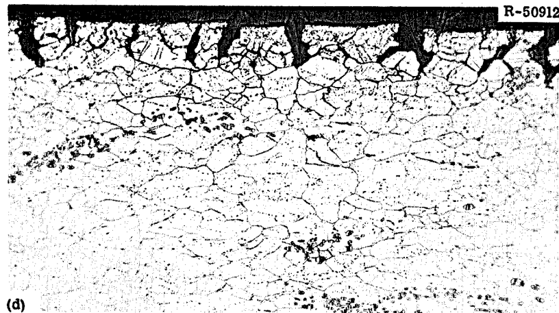
Fig. 48. Photomicrographs of a Hastelloy N (Heat 5065) Sample Tested at 25°C After Being Exposed to the MSRE Core for 22,533 hr at 650°C and Irradiated to a Thermal Fluence of 1.5 \times 10^{21} neutrons/cm 2 . (a) Fracture, etched. 100x. (b) Edge, as polished. 100x. (c) Edge, as polished. 500x. (d) Edge, etched. 100x. Etchant: glyceria regia. Reduced 26%.
