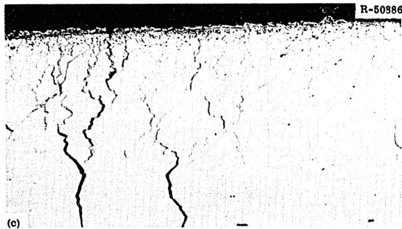
Fig. 49. Photomicrographs of a Hastelloy N (Heat 5065) Sample Tested at 650°C After Being Exposed to the Core of the MSRE for 22,533 hr at 650°C and Irradiated to a Thermal Fluence of 1.5 \times 10^{21} neutrons/cm 2 . (a) Fracture, etched. 100X. (b) Edge, as polished. 100X. (c) Edge, as polished. 500X. (d) Edge, etched. 100X. Etchant: glyceria regia. Reduced 26.5%.
