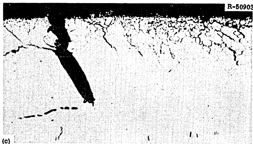
Fig. 44. Photomicrographs of a Hastelloy N (Heat 5085) Sample Tested at 25°C After Being Exposed to the MSRE Core for 22,533 hr at 650°C and Irradiated to a Thermal Fluence of 1.5 \times 10^{21} neutrons/cm 2 . (a) Fracture, etched. 100x. (b) Edge, as polished. 100x. (c) Edge, as polished. 500x. (d) Edge, etched. 100x. Etchant: glyceria regia. Reduced 27%.
