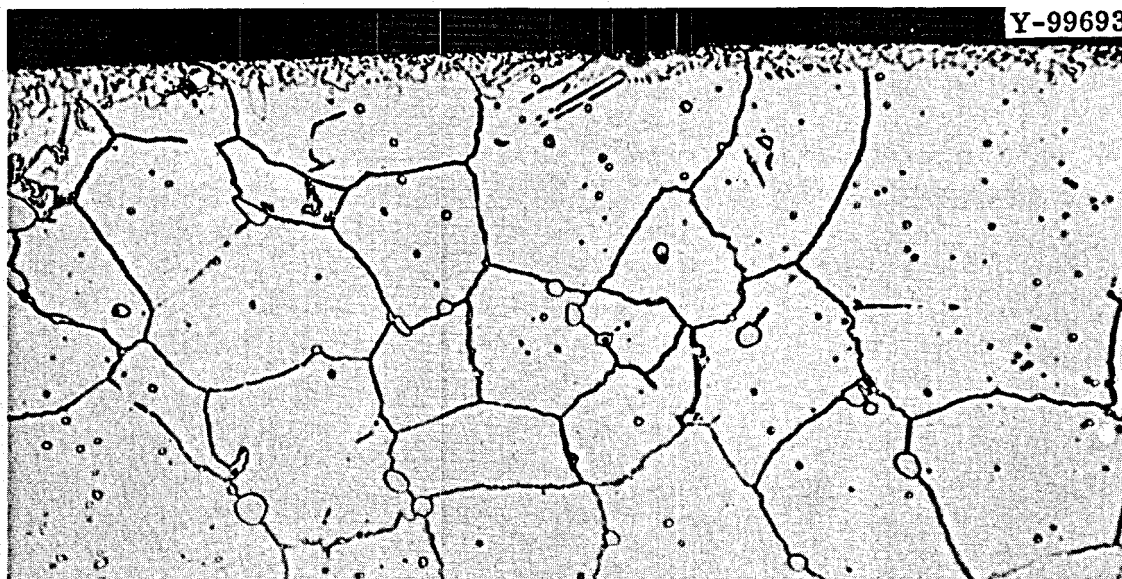
Fig. 65. Photomicrograph of Hastelloy N (Heat 5085) Rod That Was Annealed 1 hr at 1177°C, Sinterless Ground 5.2 mils, and Annealed for 4370 hr at 650°C in Argon. 500X. Etchant: glyceria regia.
