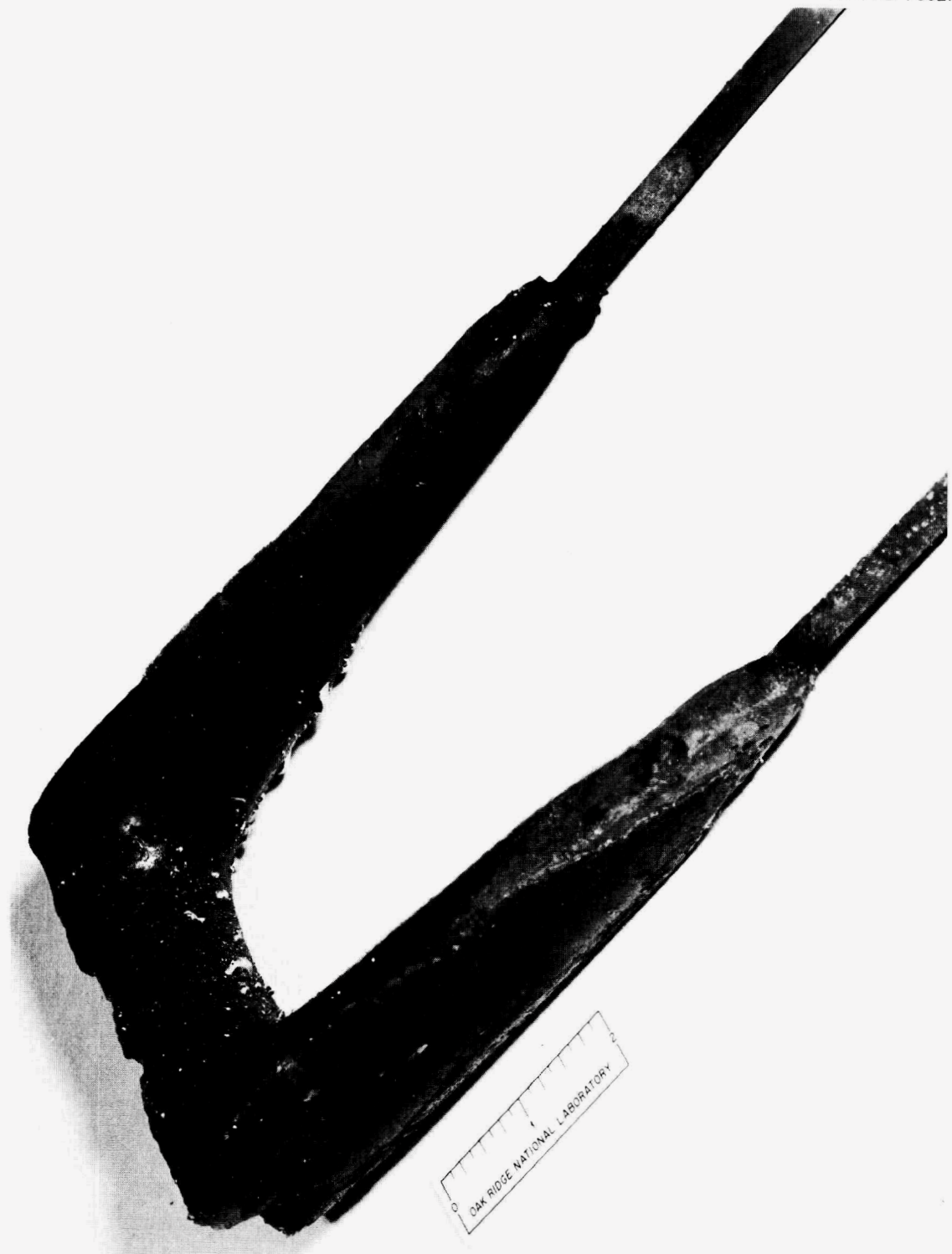
Fig. 24. Frozen Salt Film Remaining on Cooling Tube Above Quartz Electrode Divider After the Cell Vessel Cracked.
