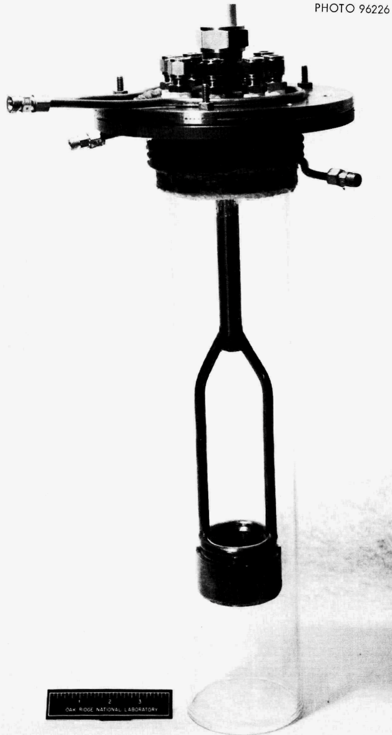
Fig. 26. Assembled Electrolytic Cell Incorporating the BeO-Insulated Anode Cup Assembly.
