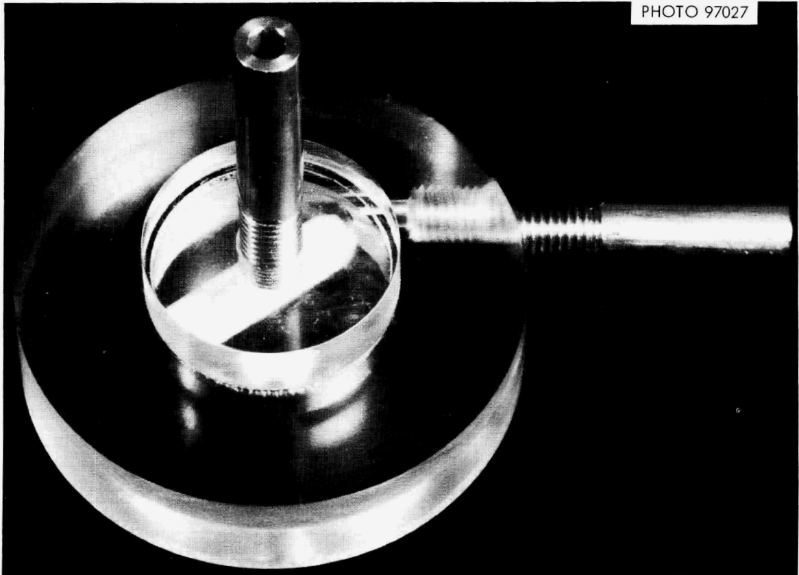
Fig. 31. Circulation Pump Used for Measurements of Axial Dispersion in Packed Columns.
