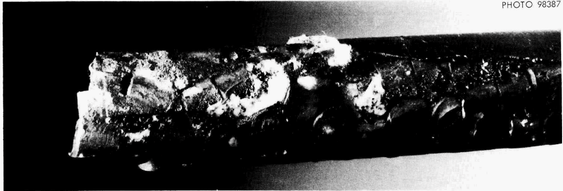
Fig. 14. Section of 0.082-in.-ID Column Showing Dendritic Iron Deposit (Upper Photograph). The lower half of the column was potted in epoxy resin, and the steel pipe was stripped away.
