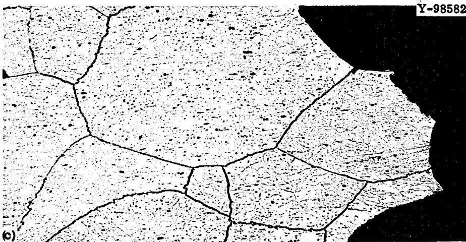
Fig. 17. Creep Fractures for Tests at 650°C and 40,000 psi in Titanium-Modified Hastelloy N for Various Heat Treatments. 100X. (a) 0.15% Ti solution annealed 1 hr at 1260°C and aged 3000 hr at 760°C, (b) 0.45% Ti solution annealed 1 hr at 1177°C and aged 1500 hr at 760°C, and (c) 1.2% Ti solution annealed 1 hr at 1260°C and aged 3000 hr at 650°C. Reduced 18%.
