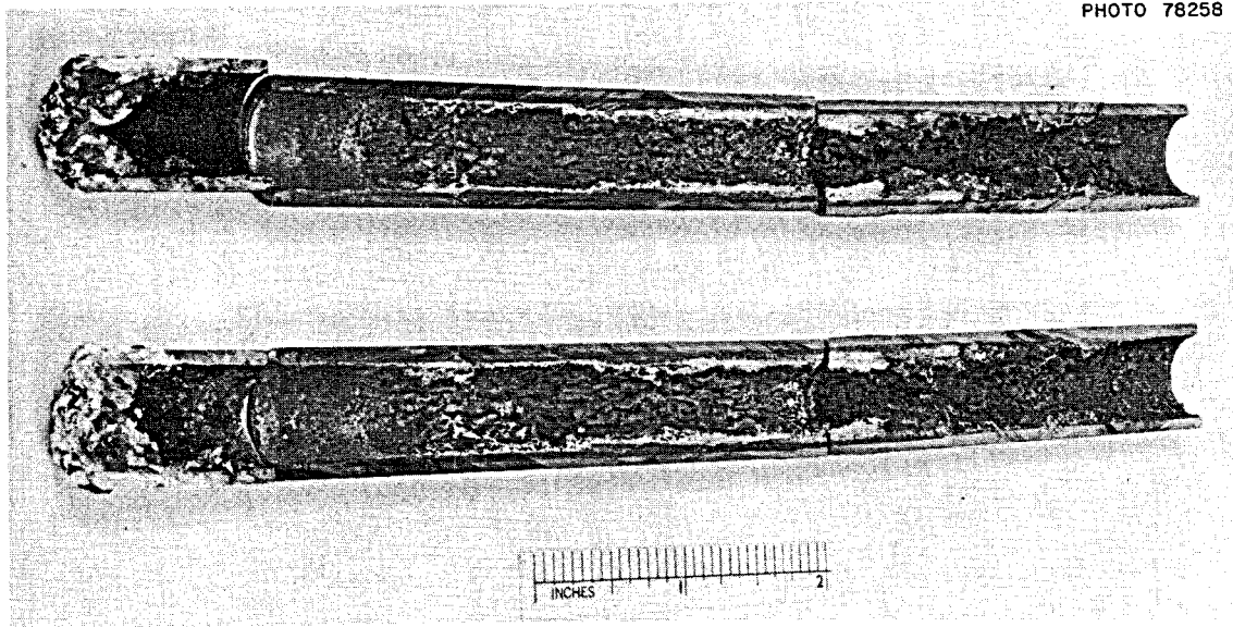
Fig. 37. Post-test appearance of salt level bubbler tube interior.
