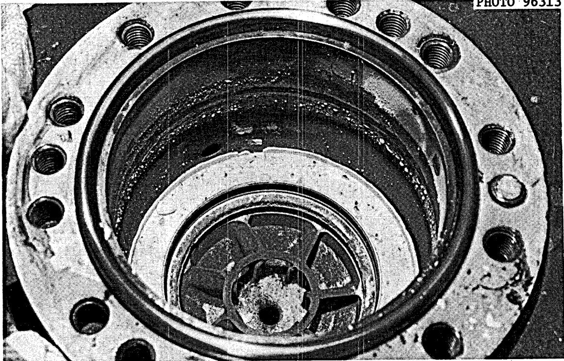
Fig. 23. Pump Bowl from Loop MSR-FCL-1. The pump operated in \text{NaBF}_4 -8 mole % NaF for 659 hr under variable conditions and 4088 hr of normal operation at 510^\circ\text{C} .
