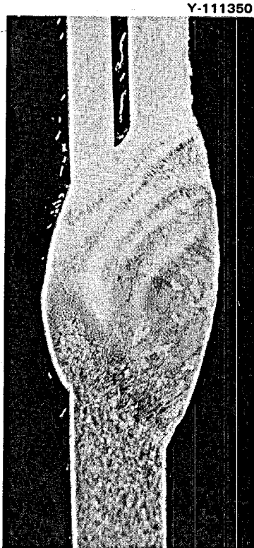
Fig. 29. Weld joining standard Hastelloy N tubing (top, right) and spacer (top, left) to modified Hastelloy N-2% Nb tubing (below). Left side exposed to salt at 665°C; right side exposed to air. Etched with glyceria regia. 12X.
