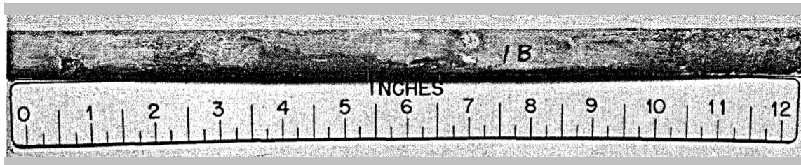
Fig. 4. Corrosive attack on exterior of Hastelloy N tubing underneath ceramic bushings after 552 hr at 675 to 785°C.
