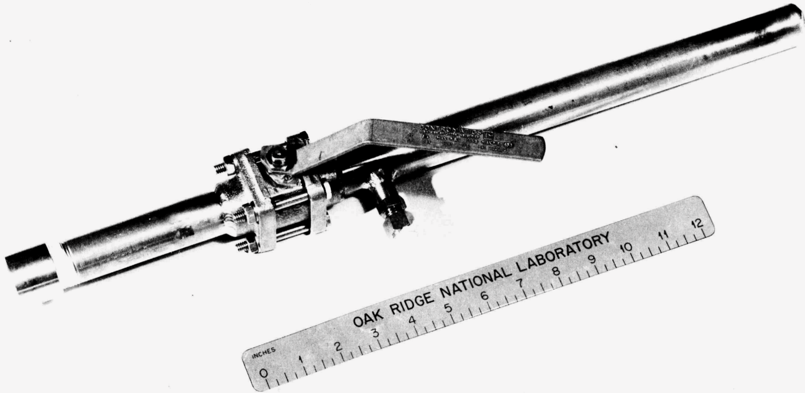
Fig. 16. Flowing stream sampler for FREE.
