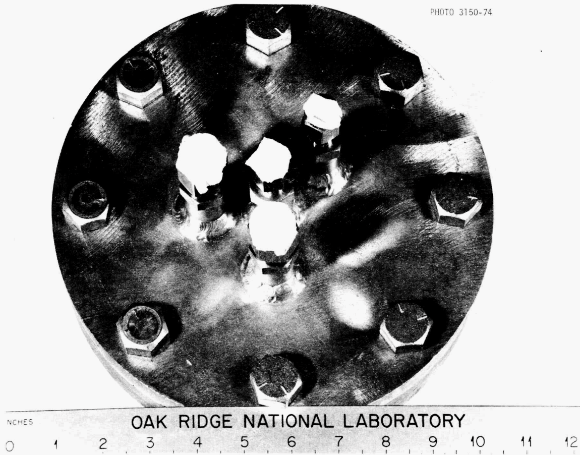
Fig. 12. Top view of UF 6 absorption vessel for FREE.
