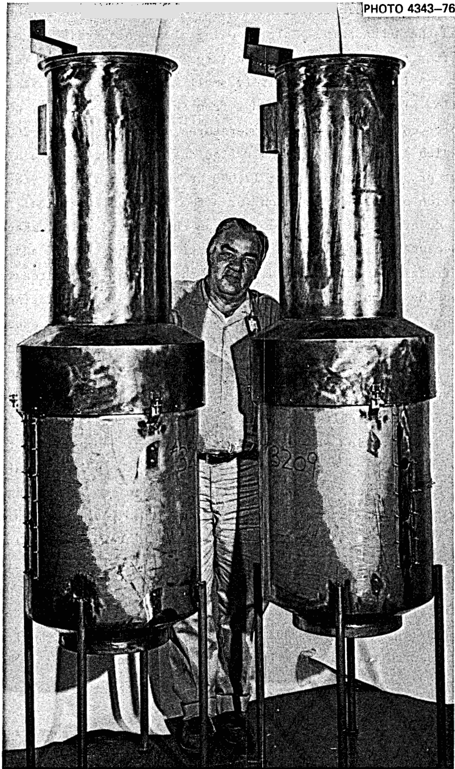
Fig. 13. Cooler housings for corrosion loop FCL-3.
